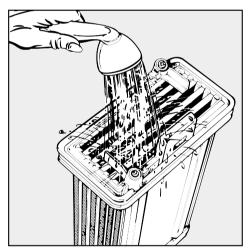
Clean the condenser unit at both ends (front and back).
